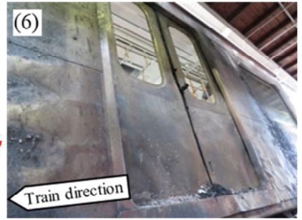
Doors for passengers damaged.
