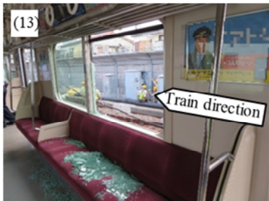
Glass in right window damaged.
