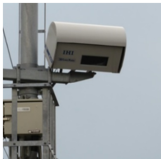
Figure 3. Laser radar head of the obstruction detecting device for level crossing
