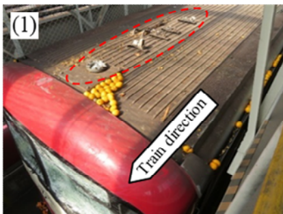
Train radio antenna damaged.
