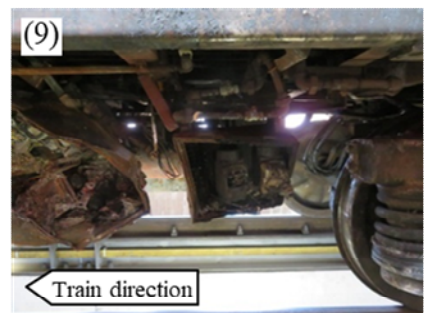
Underfloor apparatus damaged.
