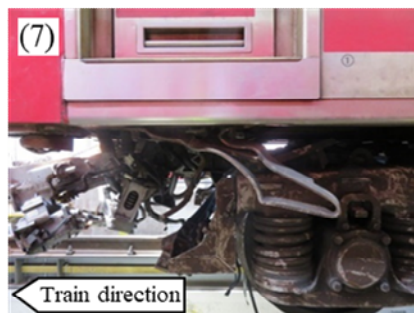
Front skirt damaged.
