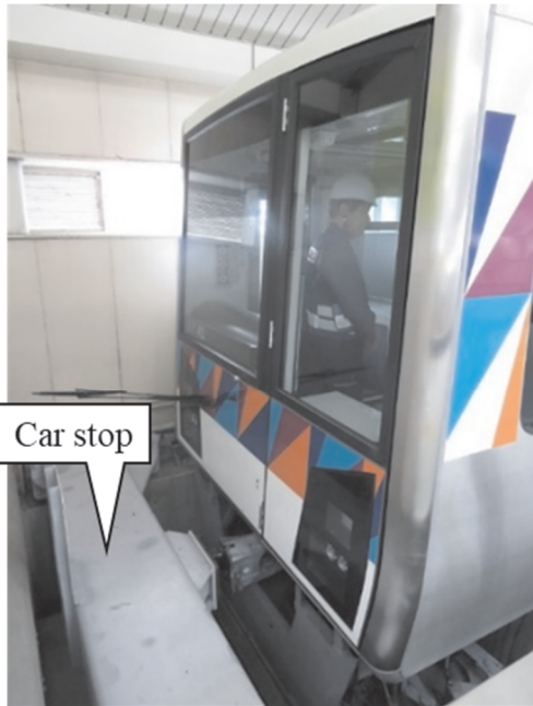
Status of collision with the car stop, the 5th vehicle
