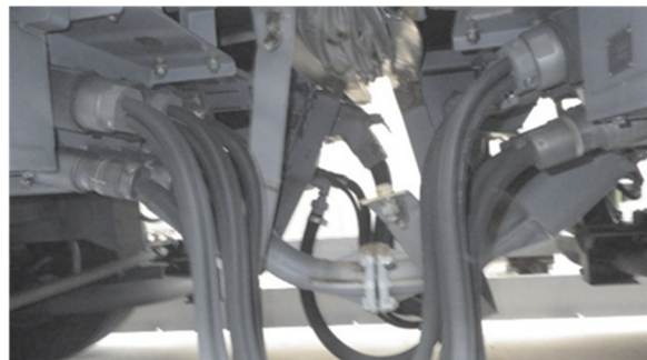
Bent intermediate coupler, between the 4th and the 5th vehicles
