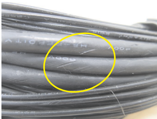
Figure 10. Flaws in the other cables
