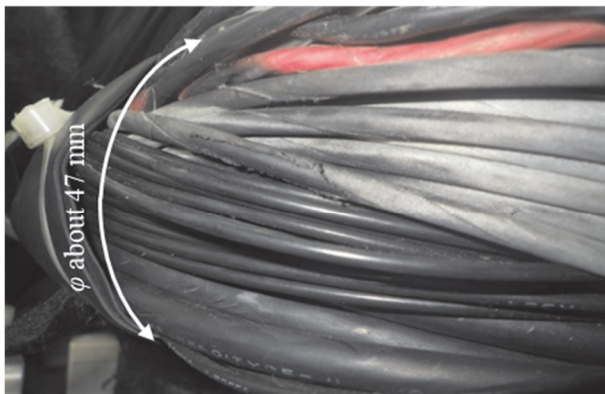
Status of electric wire, in low voltage terminal side, melted and adhered to the vehicle material.
