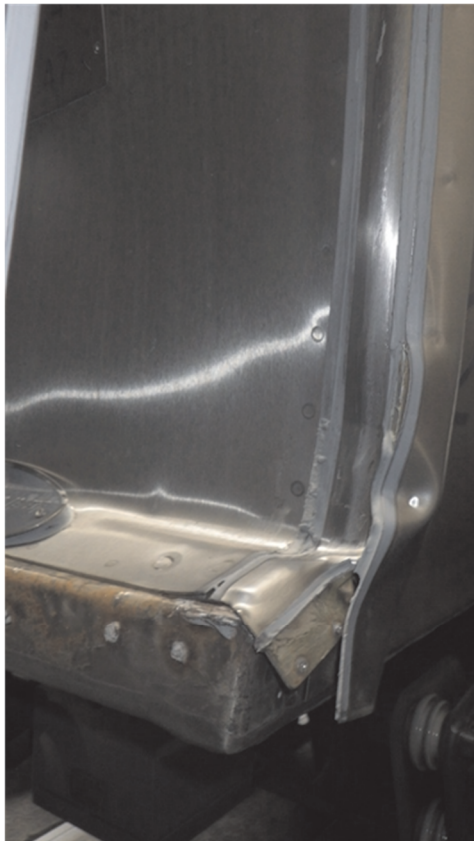
Dent of the end plate, Shin-Sugita station side of the 2nd vehicle
