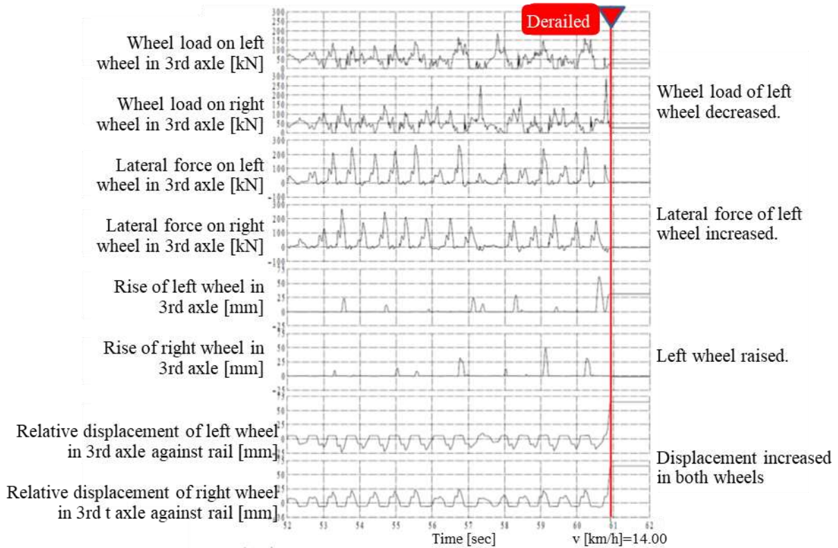
Figure 15. Results of the Simulation III (Behaviors of the 3rd Axle)
