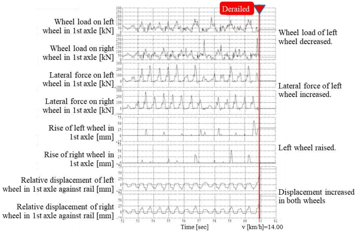
Figure 15. Results of the Simulation I (Behaviors of the 1st Axle)
