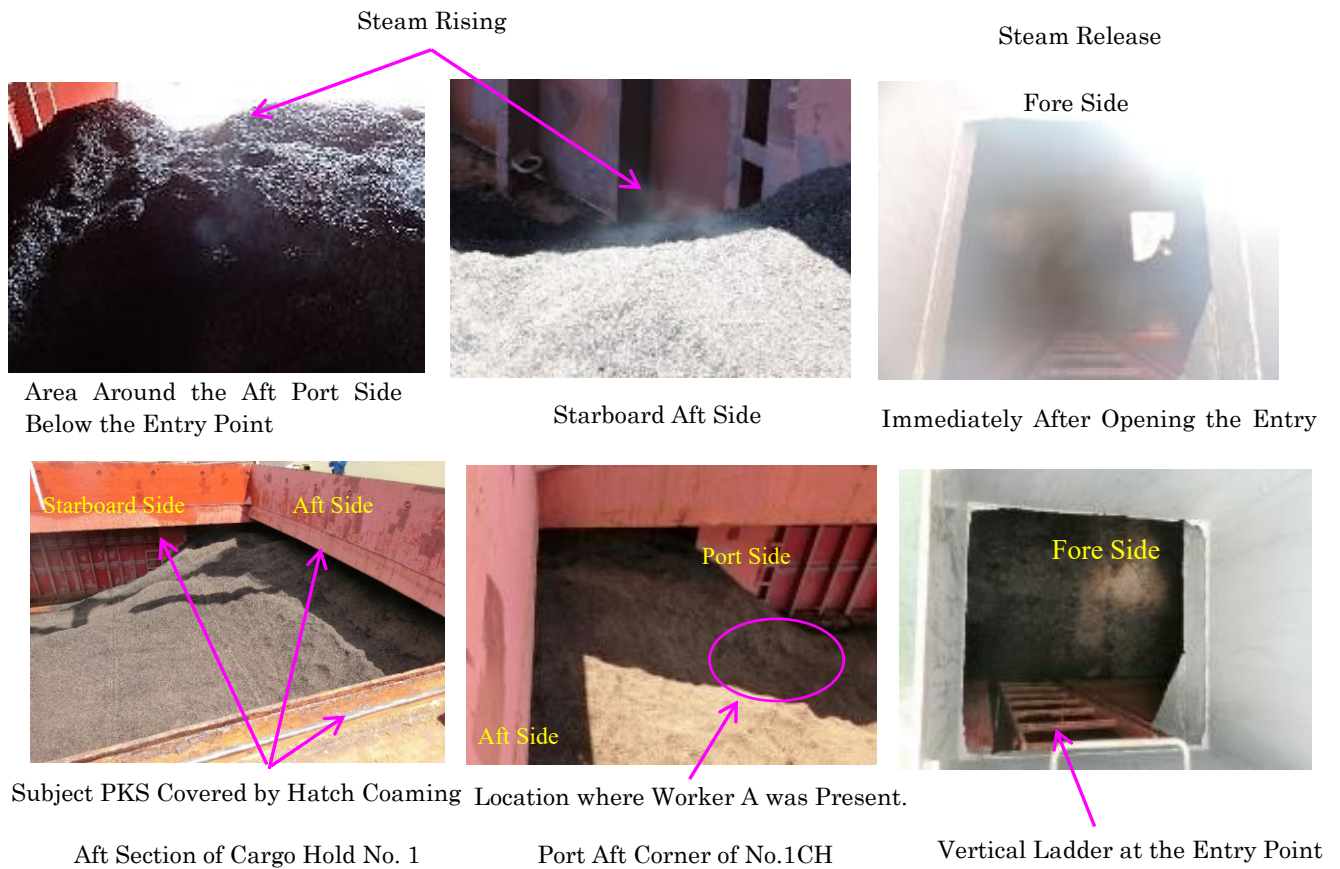
Figure 6 – Condition Inside No.1 CH (May 25)
