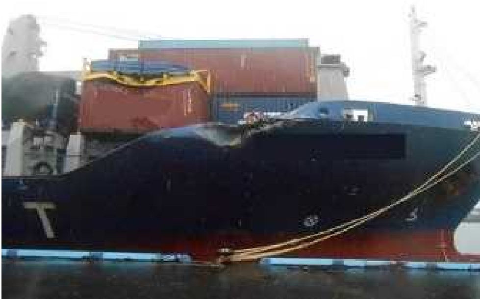
Photo 2 Status of Damage to Vessel B
