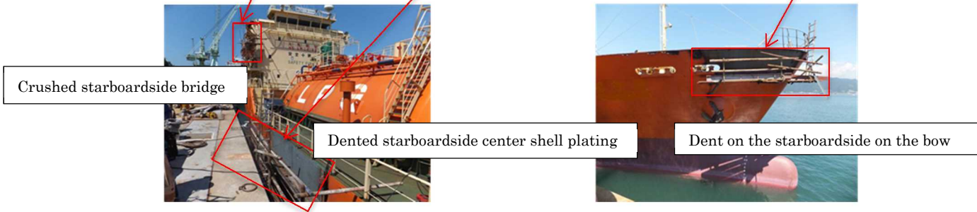
Figure 3 Damage to Vessel B
