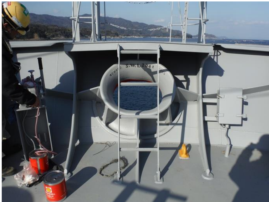
Photo 2.1-3 Vessel A's Panama Chock (Provided by Company A 1 )
