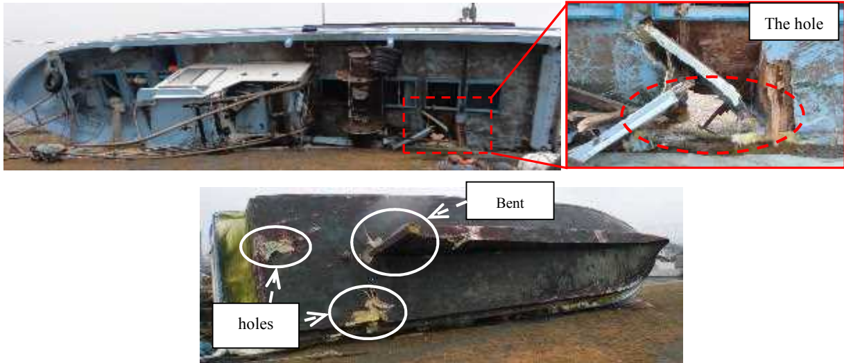
Photo 2.3-2 Damages on Vessel B
