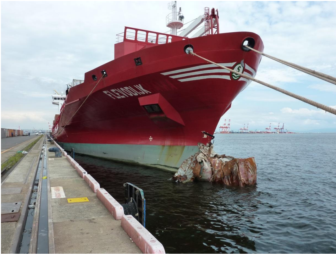
Photo 3: Damage of the Bulbous Bow
