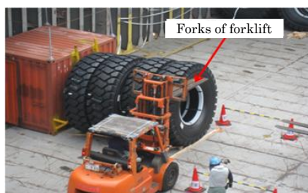
Photo 6 Tire Fall Prevention by Forklift – Example 1
