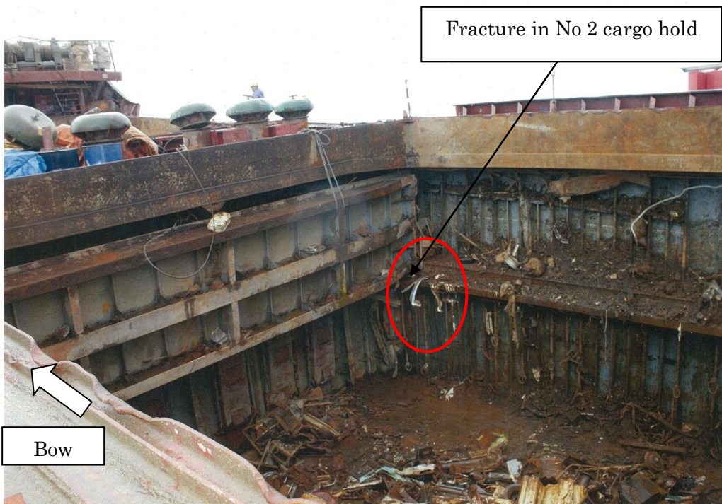
Photo 6 Damage to Vessel B (2) (Conditions after being salvaged)
