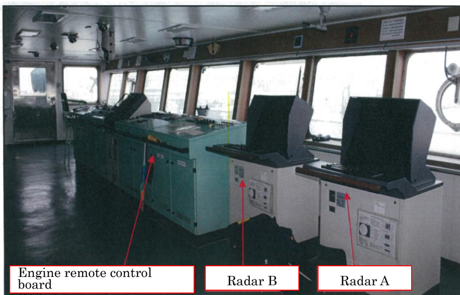
Photo 2.1-3 Inside of the bridge on Vessel A
