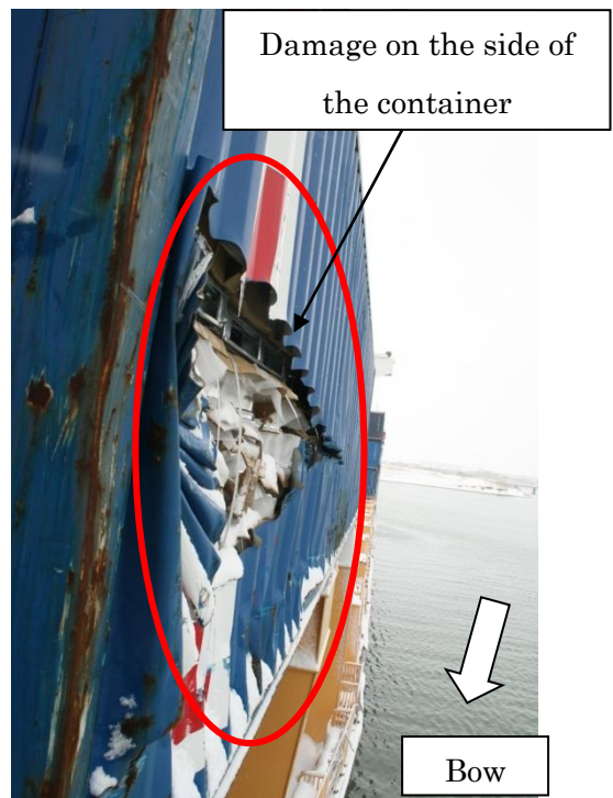
Photo 3 Damage to Vessel A (3)
