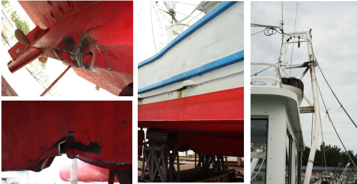
“Damage to Vessel B” (Left: a buckling and a fracture to the keel, Center: a dent to the shell plating at the central part of the starboard side, Right: a bent to the mast for drawing a fishing net)
