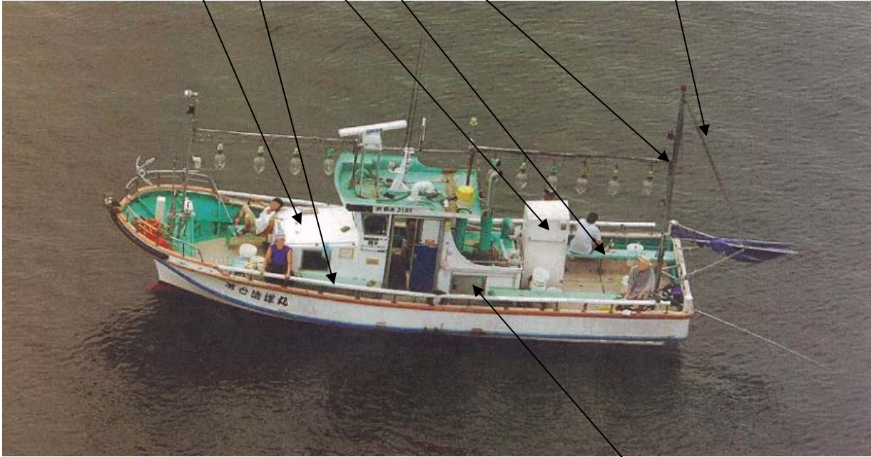
Sliding door of engine room
