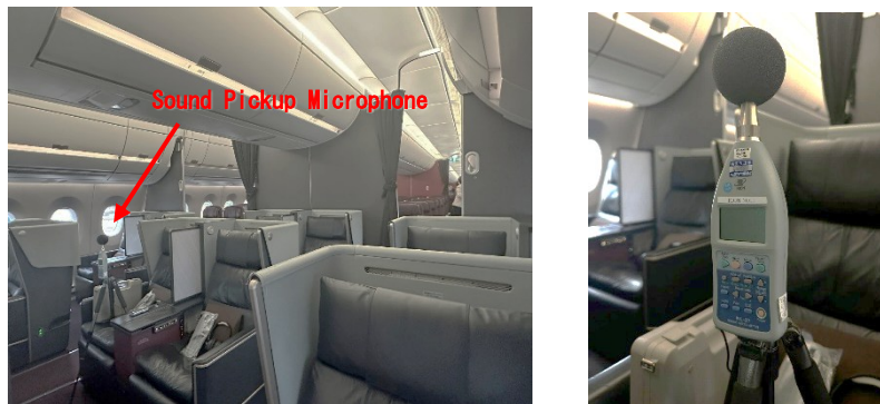
Figure 7: Sound Pickup Microphone Used During the Verification Experiments
