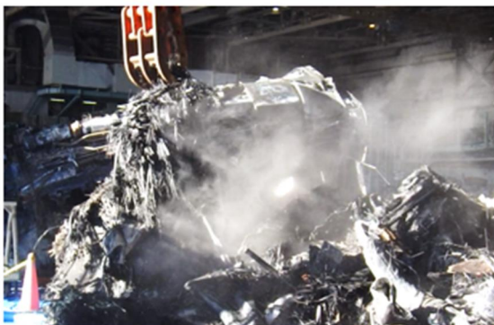
Figure 34-2 Dust after CFRP Burnout
