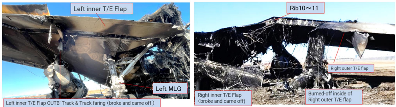
Figure 35: Condition of the Main Wing (from rear)
