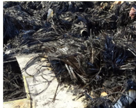
Figure 34-1: Burnout of the CFRP of Aircraft B (Left: underside of the right main wing, Right: fuselage)
