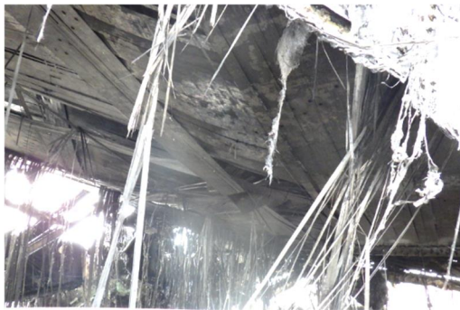
Figure 34-1: Burnout of the CFRP of Aircraft B (Left: underside of the right main wing, Right: fuselage)
