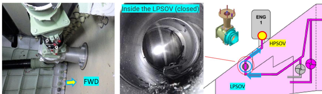
Figure 50-3 : Left LPSOV Status after the Event (additions to the drawing provided by Airbus)
