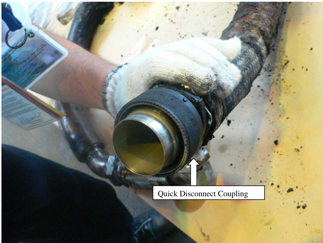
Photo 6 Fuel Supply Hose Coupling (Inserting)
