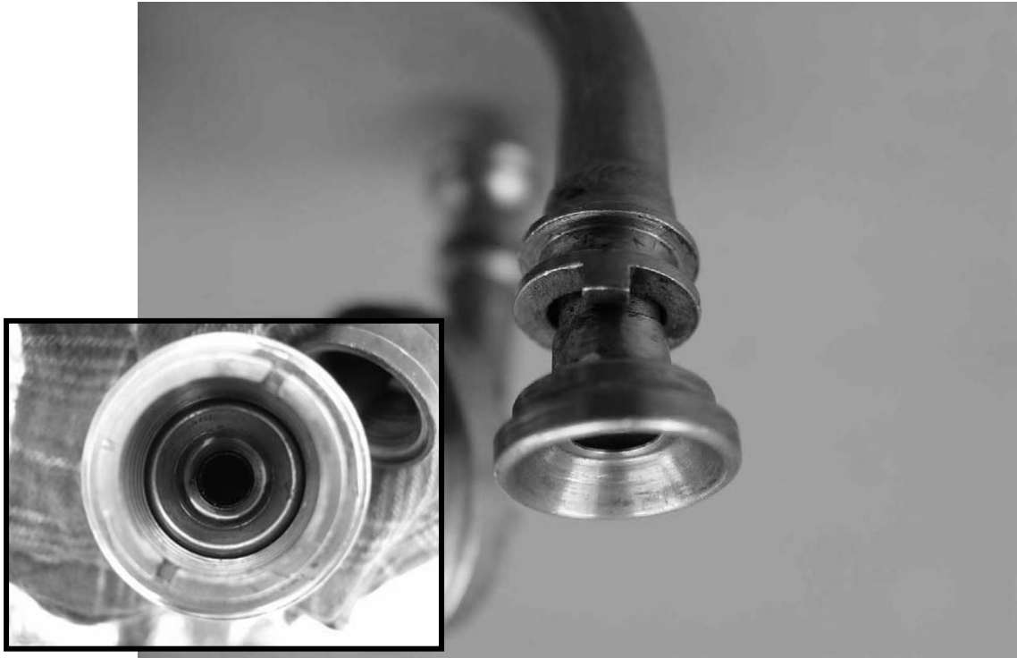
Photograph 6 Leak check at Primary Fuel Tube attachment area connecting to No.3 Fuel Nozzle
