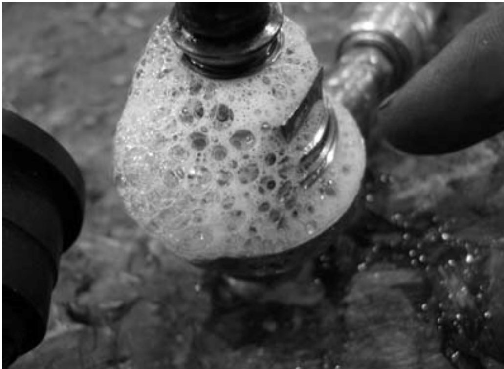
Photograph 6 Leak check at Primary Fuel Tube attachment area connecting to No.3 Fuel Nozzle
