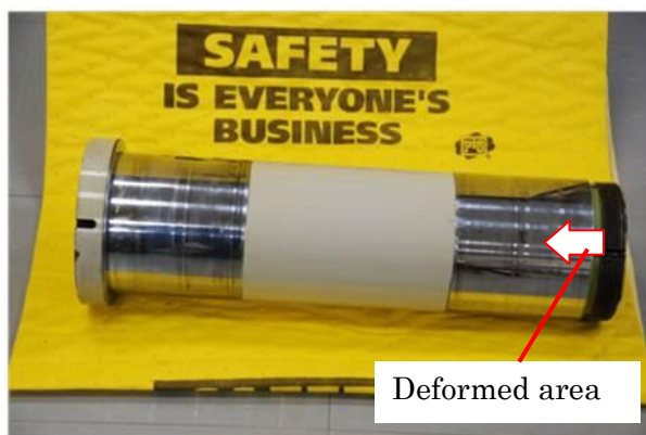
Photo 17 Track Beam Bolt
