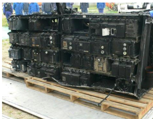
Photo 15 Removed Avionics Rack
