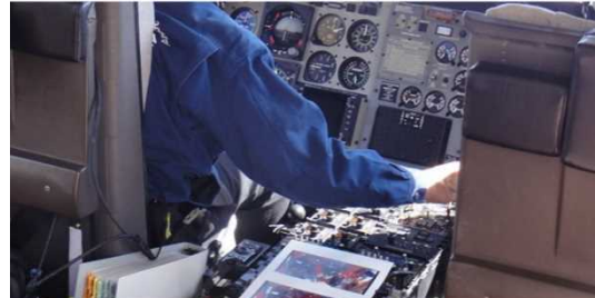
In the inspection (operating the ITT trim switch with the CP lever moved to the position at the time of climbing)
