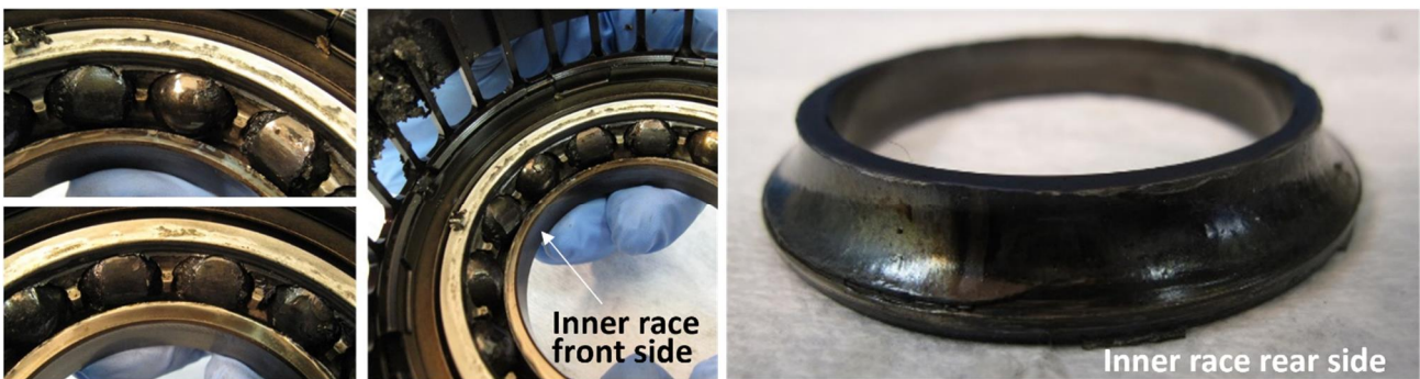
Figure G: Damage to No.1 Bearing
