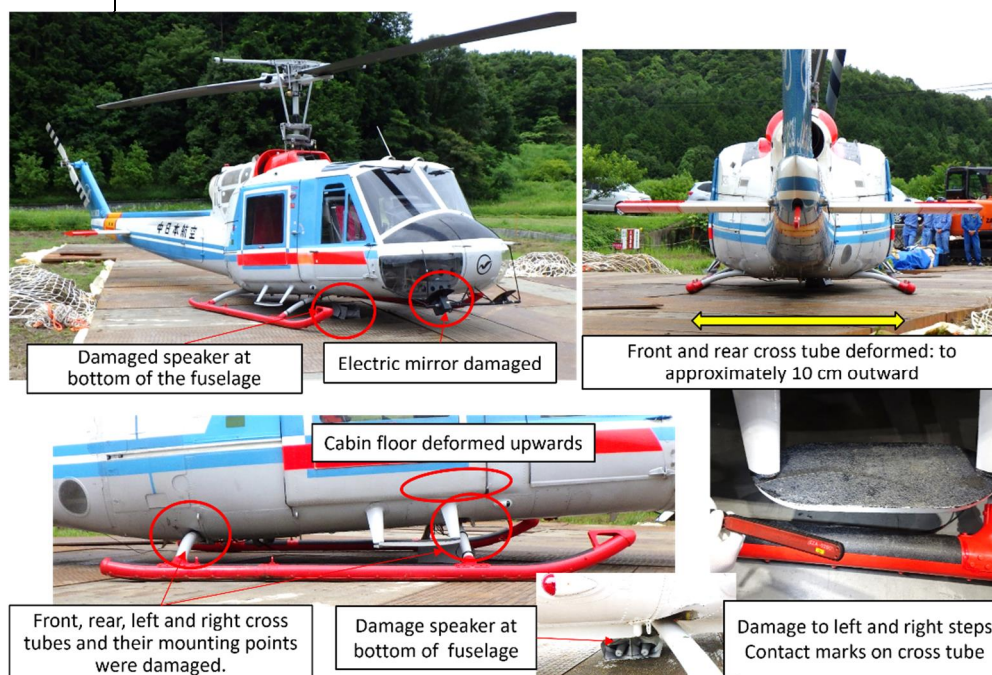
Figure 4: Damage to the helicopter and its touchdown conditions
