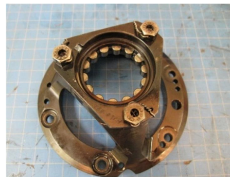
Figure I: No.21 Bearing condition
