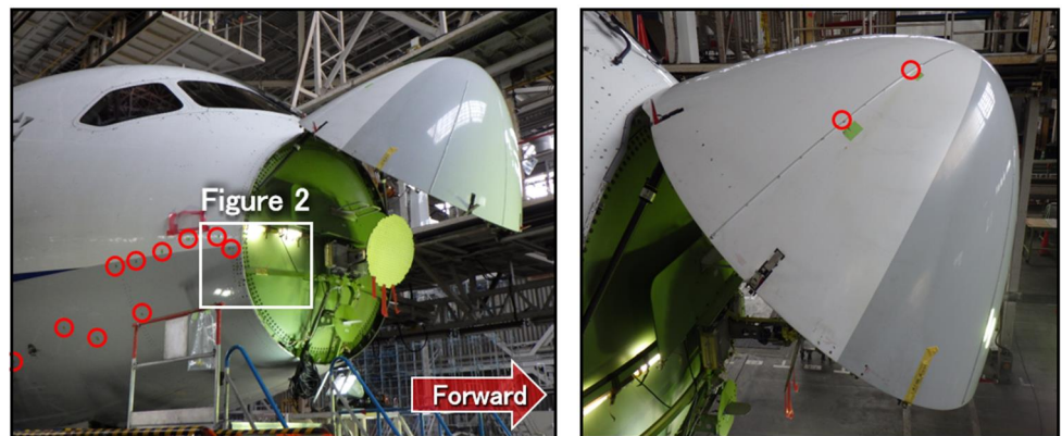
Figure 3: Damage to Parts other than those Requiring Major Repairs
