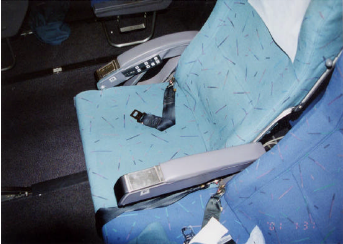
Damage of seat armrest of right side pass way seat No. 33
