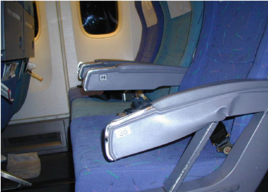
Damage of seat armrest of right side pass way seat No. 35
