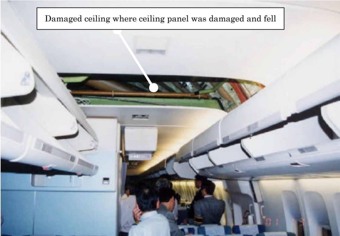
The damage of ceiling panel over left side pass way seat No. 41(view from front)
