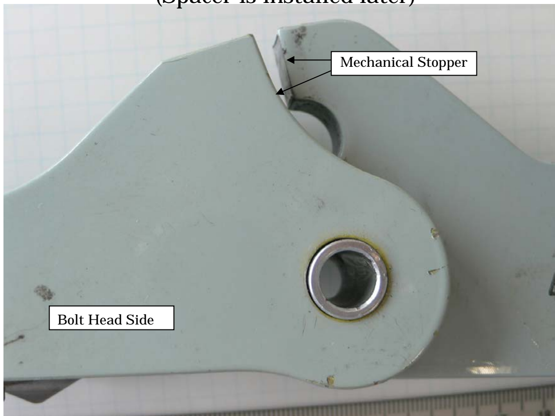
Photo 7 Toggle-Link removed from the accident aircraft (2) (Spacer is installed later)
