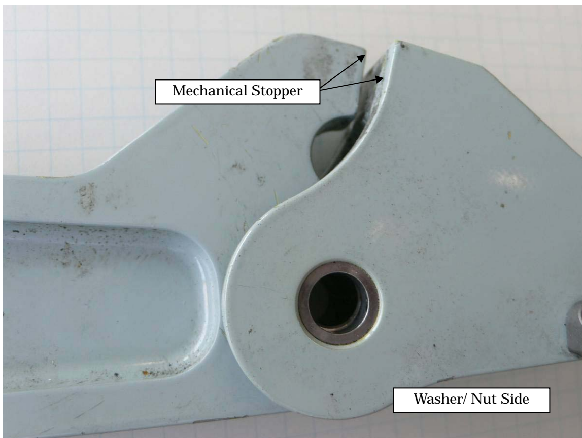
Photo 8 Toggle-Link removed from the accident aircraft (3)
