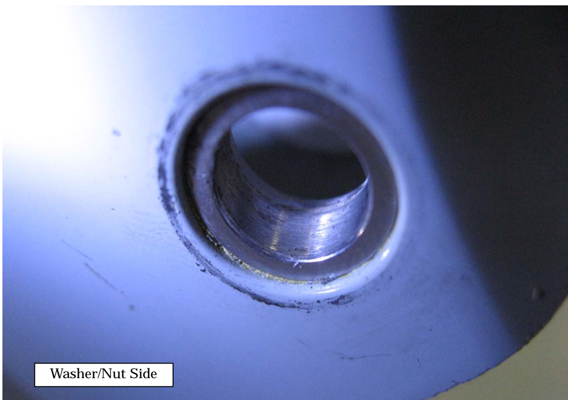
Photo 13 Inner Surface of Flanged Bushing removed from aircraft D
