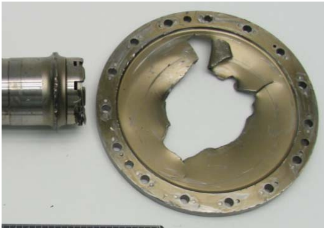
Photo 4 Fracture situation of RGB input shaft
