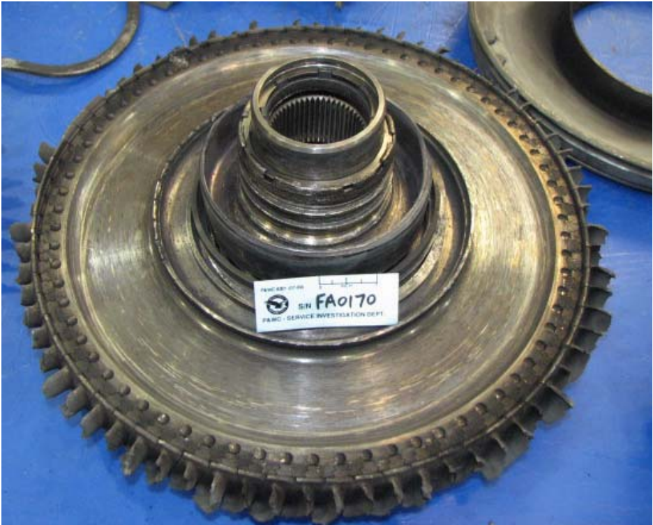
Photo 11 Fractured PT blade
