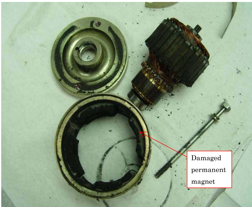
Photo 15 Damaged motor of feathering pump
