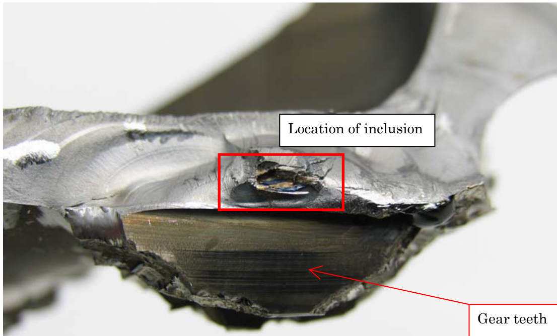
Photo 7 Extended figure of initial crack
