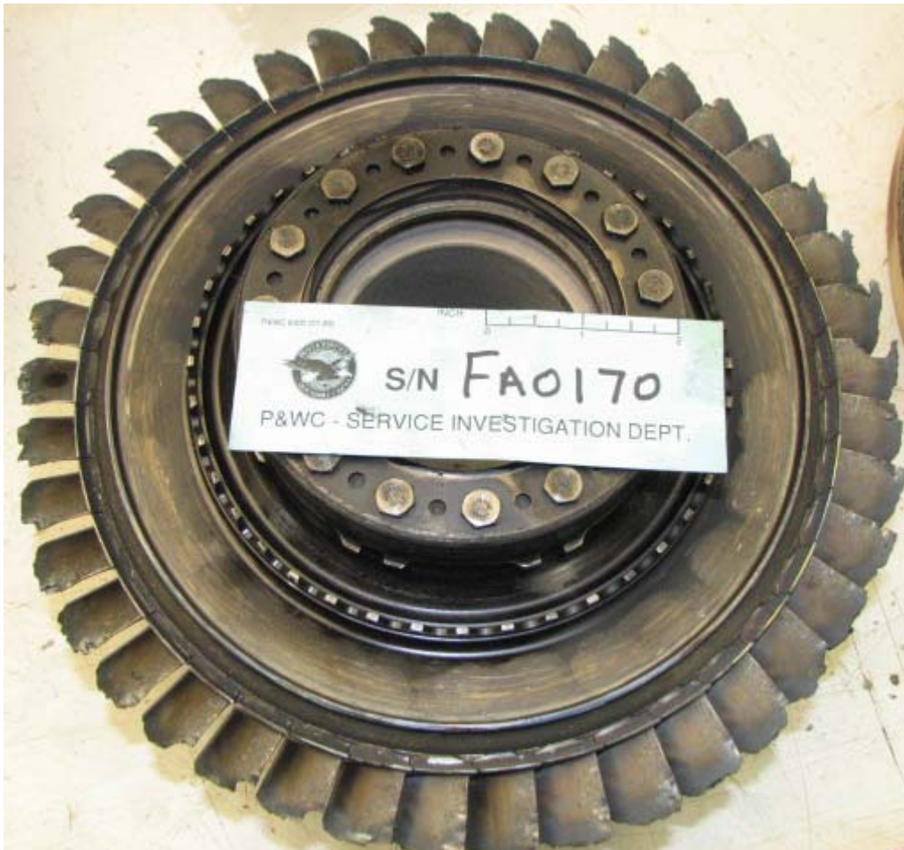
Photo 12 Damaged HPT blade
