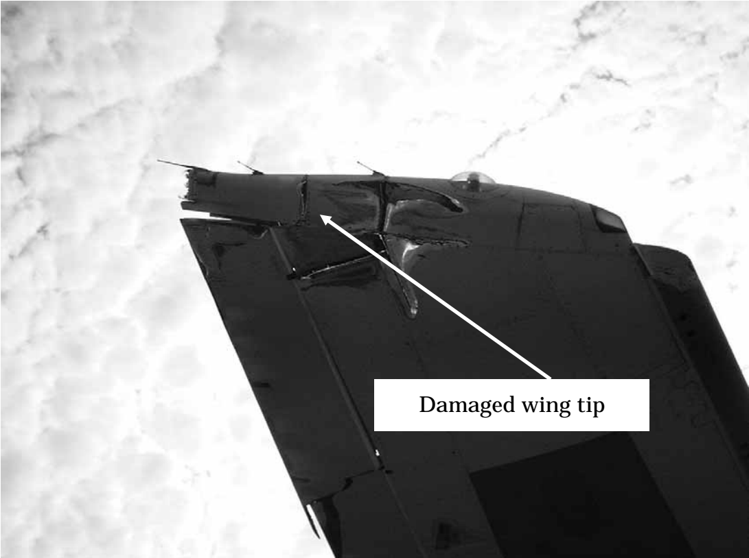
Photograph 4 Damages of the right wing
