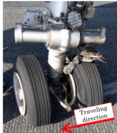
Figure 2: Damages to the nose landing gear
