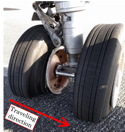
Figure 2: Damages to the nose landing gear
