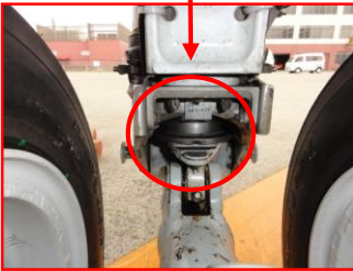
Undamaged part of the same type aircraft (Piston cap)
