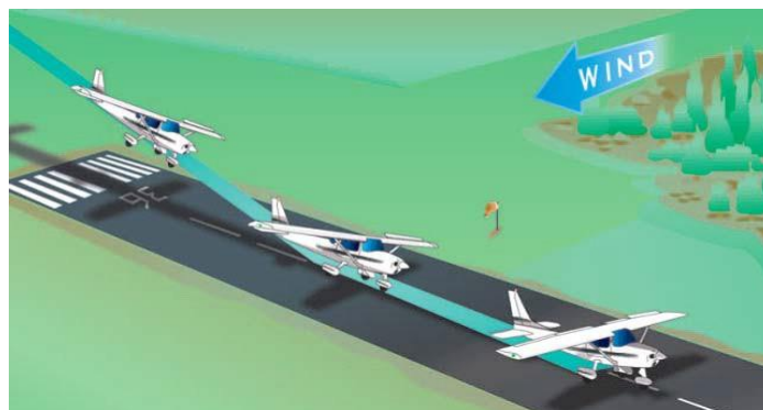
Diagram 3 : Crosswind landing (first touch down is with the main landing gear of the windward side) 「Airplane Flying Handbook」 (Fig. 8-17)
