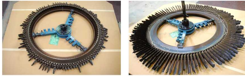
Figure 4: Damaged condition of LPT fifth stage disk and blades (left) and sixth stage disk and blades (right)
