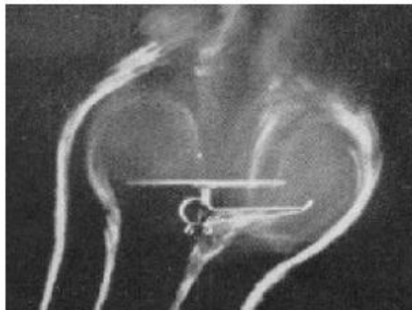
Figure 1. Smoke flow visualization of a rotor in vortex ring state (Dress, ref. 20).
