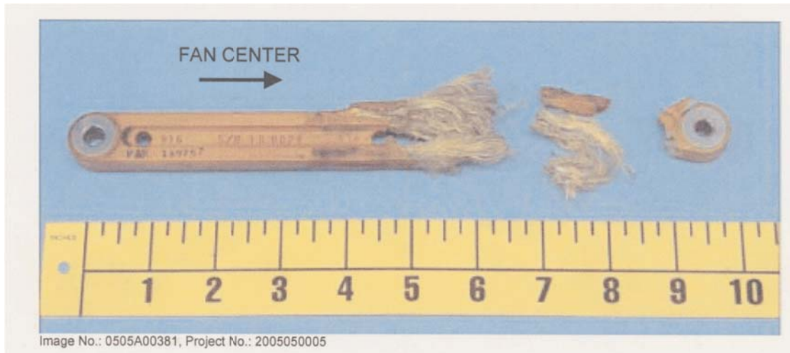
Picture A Fractured T-T strap
