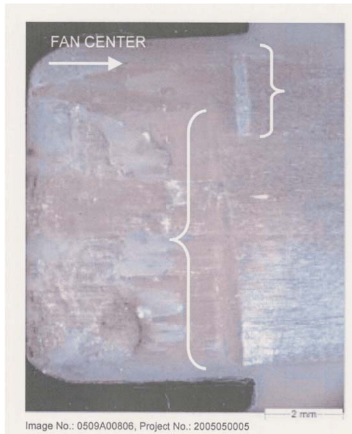
Picture G Close view of fiber kinking
