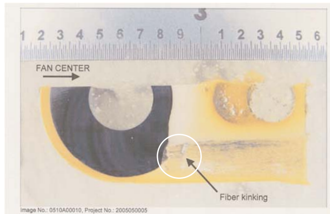
Picture D Cross section in a plane nearly perpendicular to the spool axis
