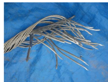
(Photo 3: Fracture surface of an electric wire)
