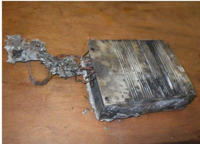
Strobe light power supply and its wires investigated by NTSB
