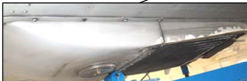
Damaged anti-collision light and air-conditioner condenser
