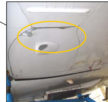
Damaged LH main landing gear door
