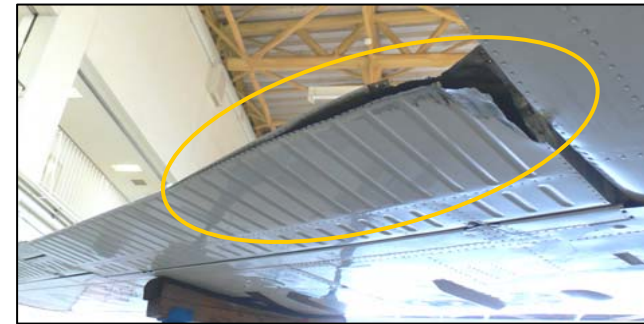
Damaged LH flap
