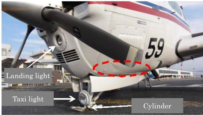
Photo 2: State of Damage to Various Parts
