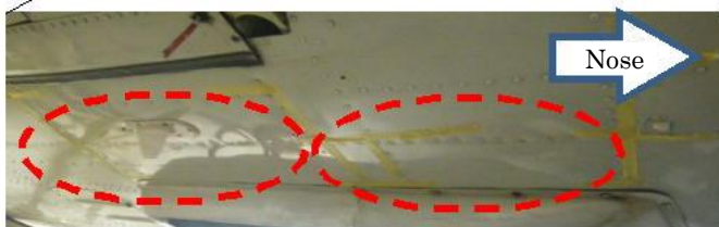
Wrinkling on lower outer plate in center of fuselage
