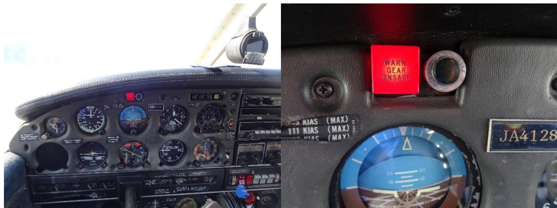
Figure 2: Landing Gear Warning Light (Illuminated State)
