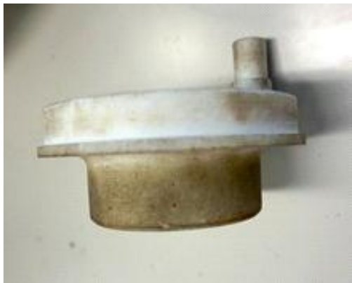
Photo #24: Butt part of propeller blade created by 3D printer
