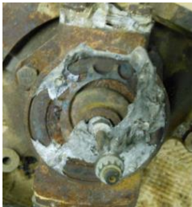
Photo #5 Remains of compressor wheel
