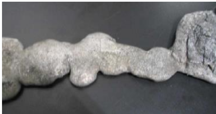
Photo – Melted Propeller Blade
