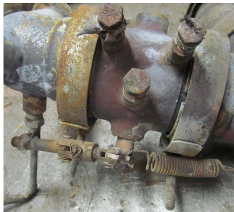
Photo #1 – Wastegate valve
