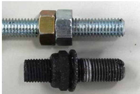
Photo #25: Low Pitch Stop Bolt (bottom) and Substitute Bolt (top)
