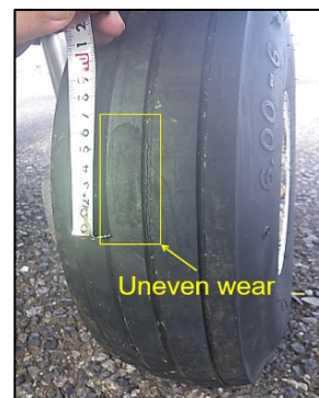
Figure 6: Left main landing gear wheel
