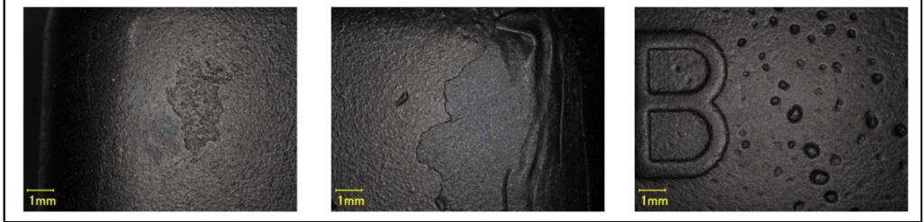
Figure 10 Uneven surfaces of foamed portion (representative portions)
