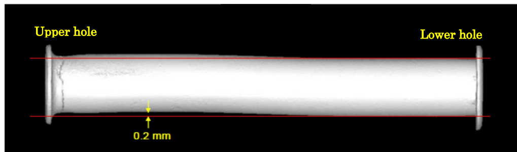
Figure 9 Warped insert in abnormal float
