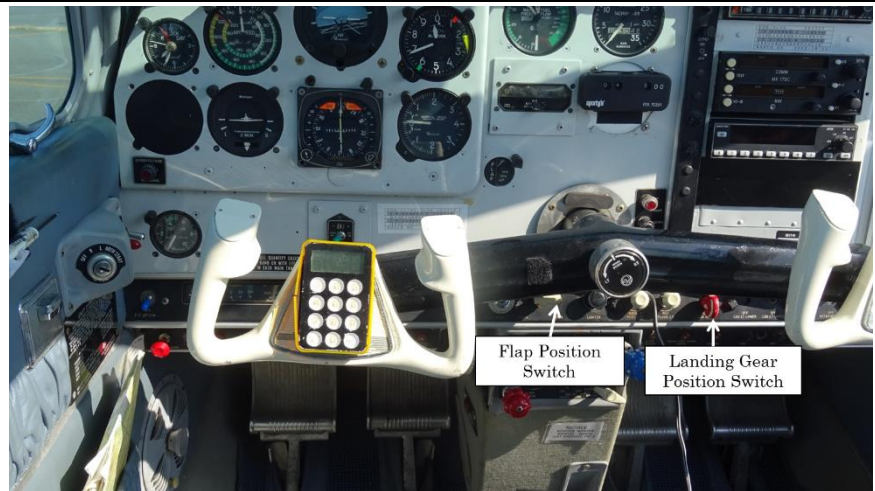
Photo 3 Location of Flap position switch and Landing gear position switch
