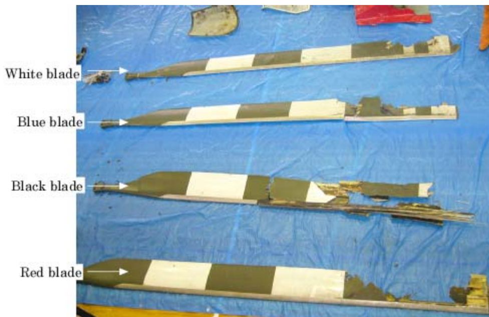
Photo 4 Damaged Main Rotor Blades
