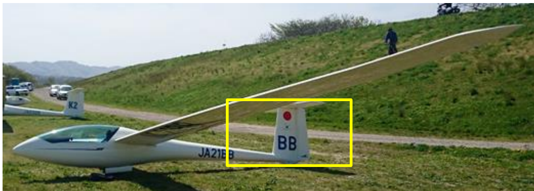
Photo K Separated after fuselage including the tail (state before the accident)
