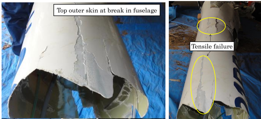
Photo M State of the upper forward fuselage
