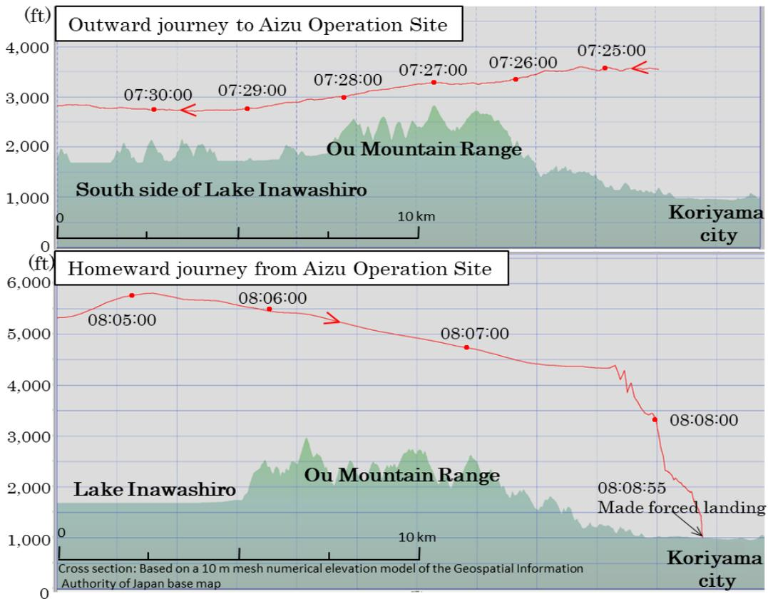
Figure 2: Cross-sectional view during the helicopter's flight over the Ou Mountain Range
