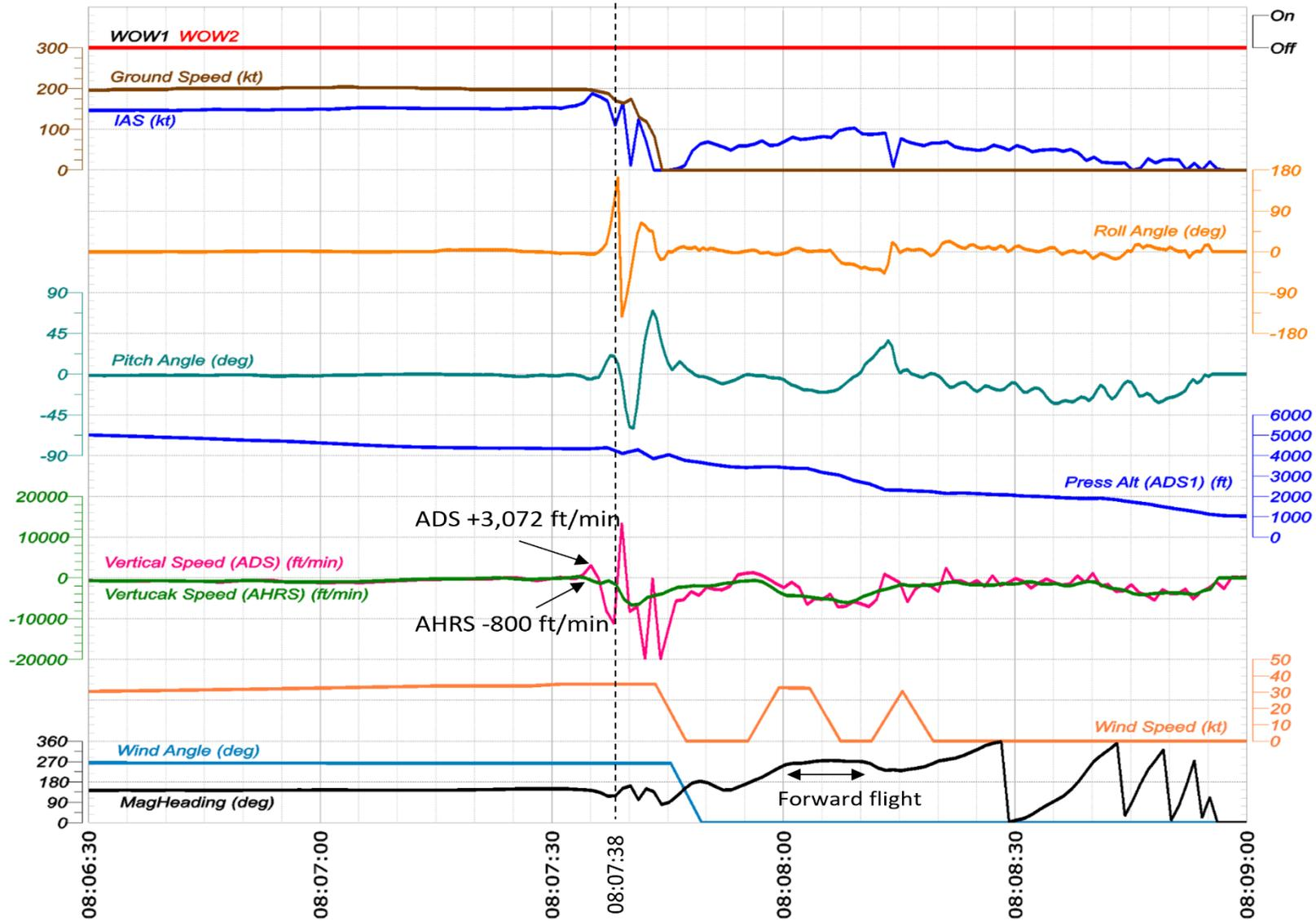
Appended Figure 5: MPFR Analysis before and after right rolling motion - 2
