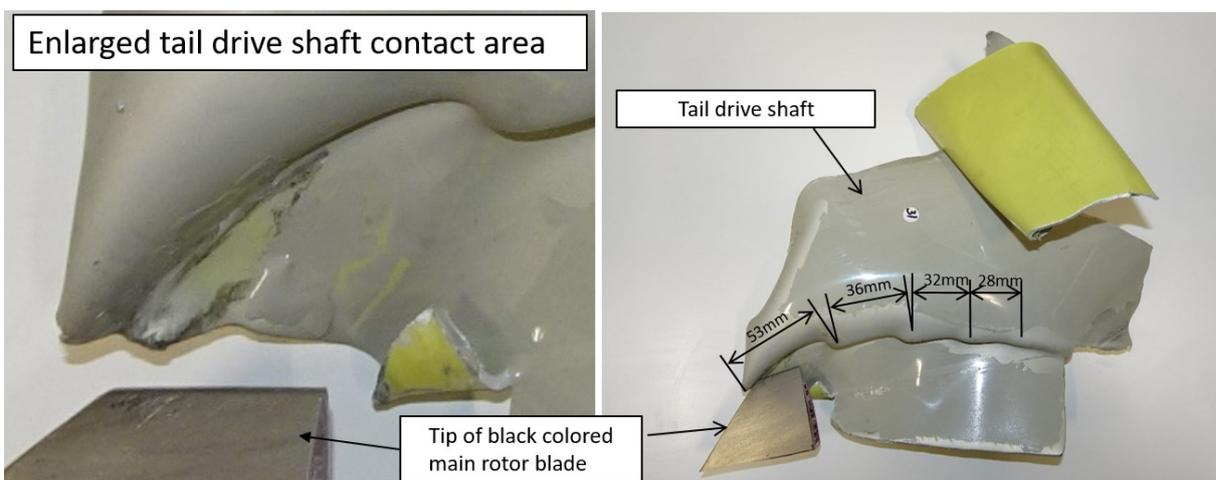
Figure 15: Contact marks between black main rotor blade tip and tail drive shaft
