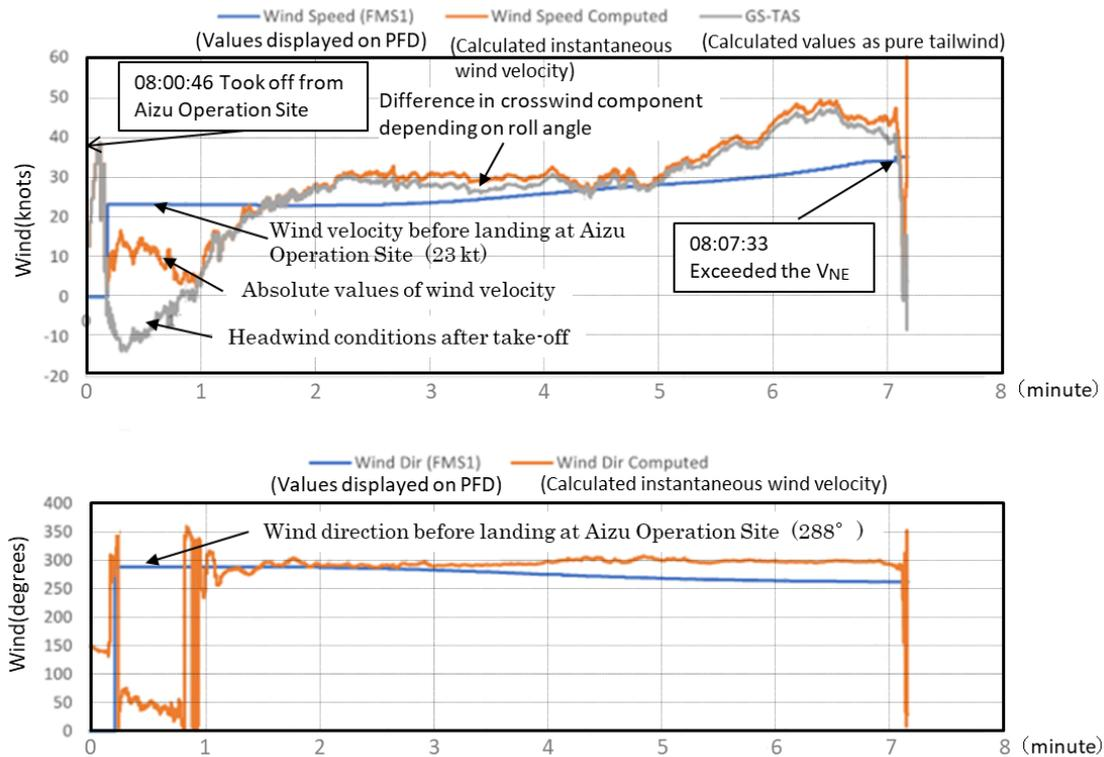
Figure 17: Comparison between the winds computed by FMS and the instantaneous wind
