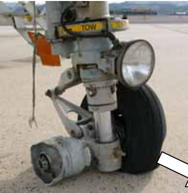
Photo 4 Damaged Nose Gear
