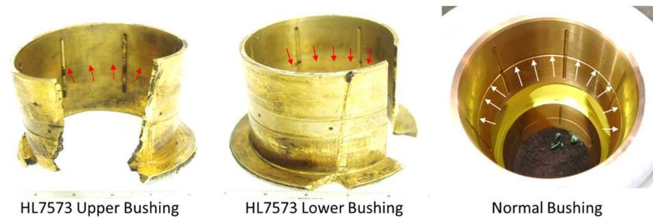
Figure 15 Circumferential grease groove on Bushing ID
