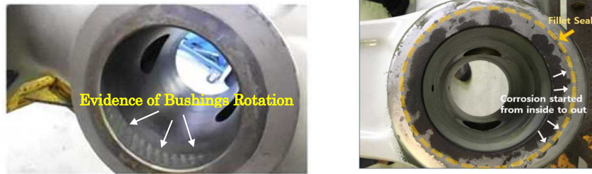
Figure 16 Axle Pivot of the Same Type of the Aircraft (after removing bushing)
