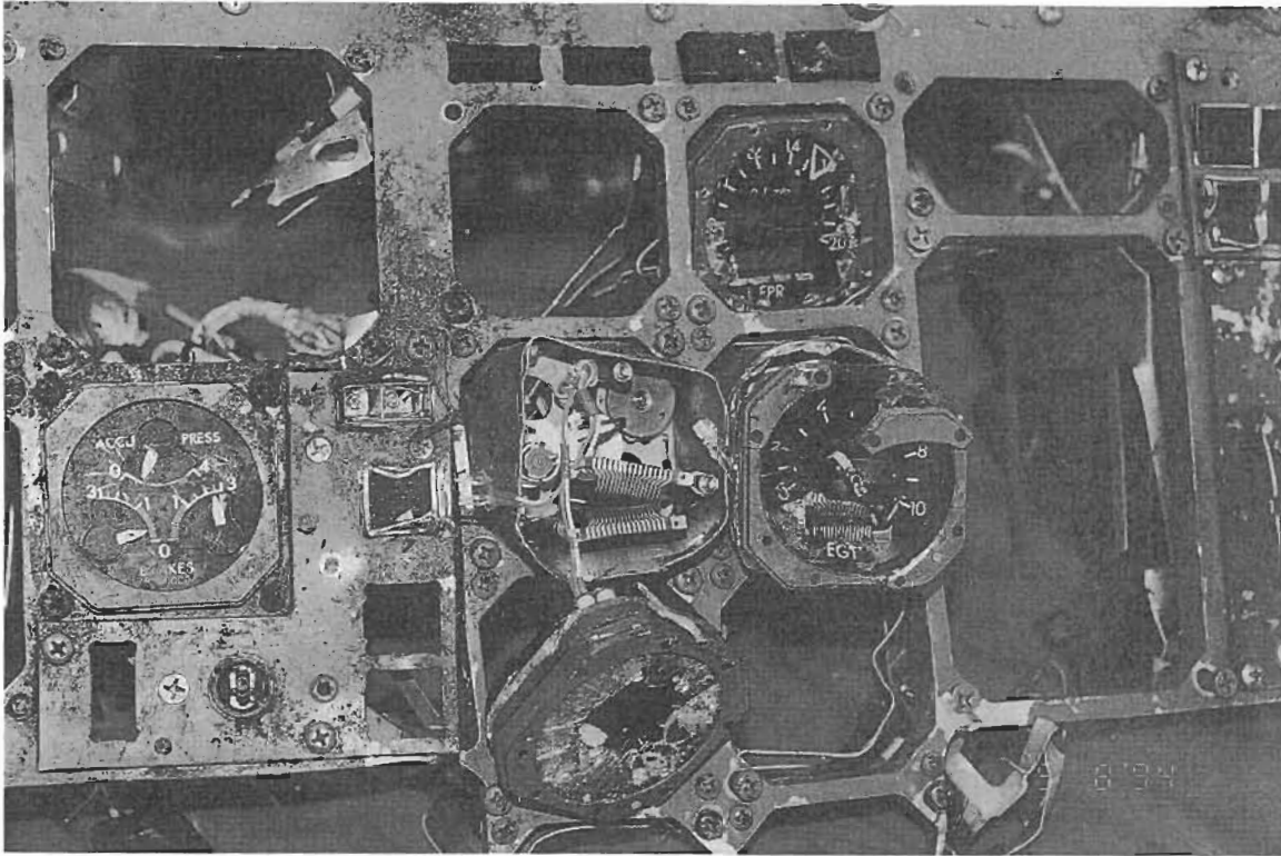
Photo.41 Outward Appearance of Display Unit with Broken Indicators
