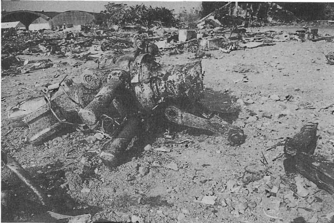
Photo.25 Leg Assembly of the Nose Landing Gear
