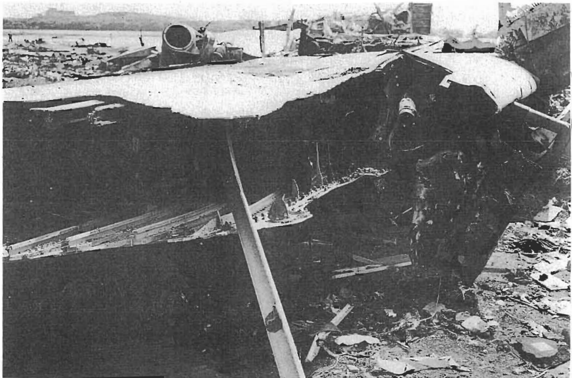
Photo.20 Fractures of the Right Wing
