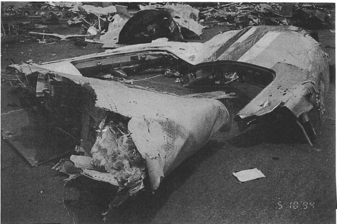
Photo.28 Part of Outside Surface of the R1 Door
