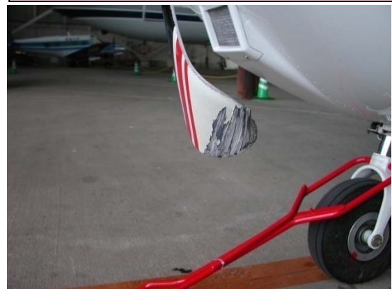
Damage of the propeller blades
