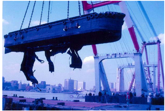
Vessel B which Sustained a Fracture at the Bottom
