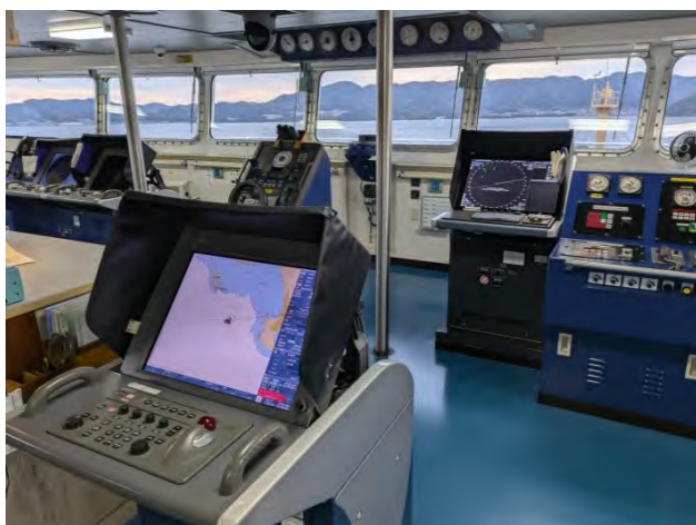
Bridge of the training ship "Taisei Maru" (Lower left: ECDIS, Upper right: Radar/ARPA)
