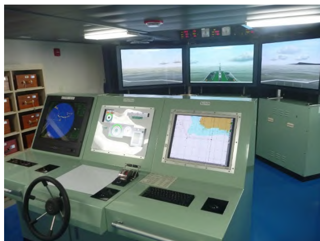
Ship Simulator installed on the training ship bridge on the lower deck
