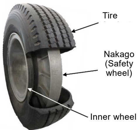
An example of a running wheel being used on the new transportation system
